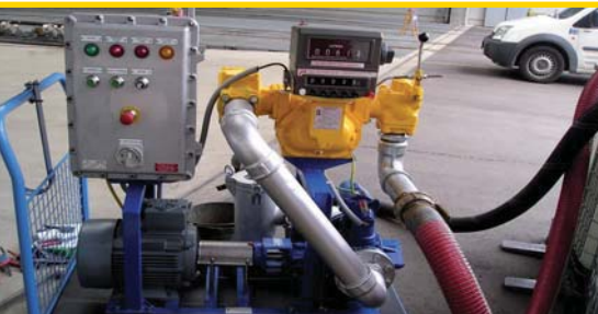
Mobile ATEX deloading system with counter
